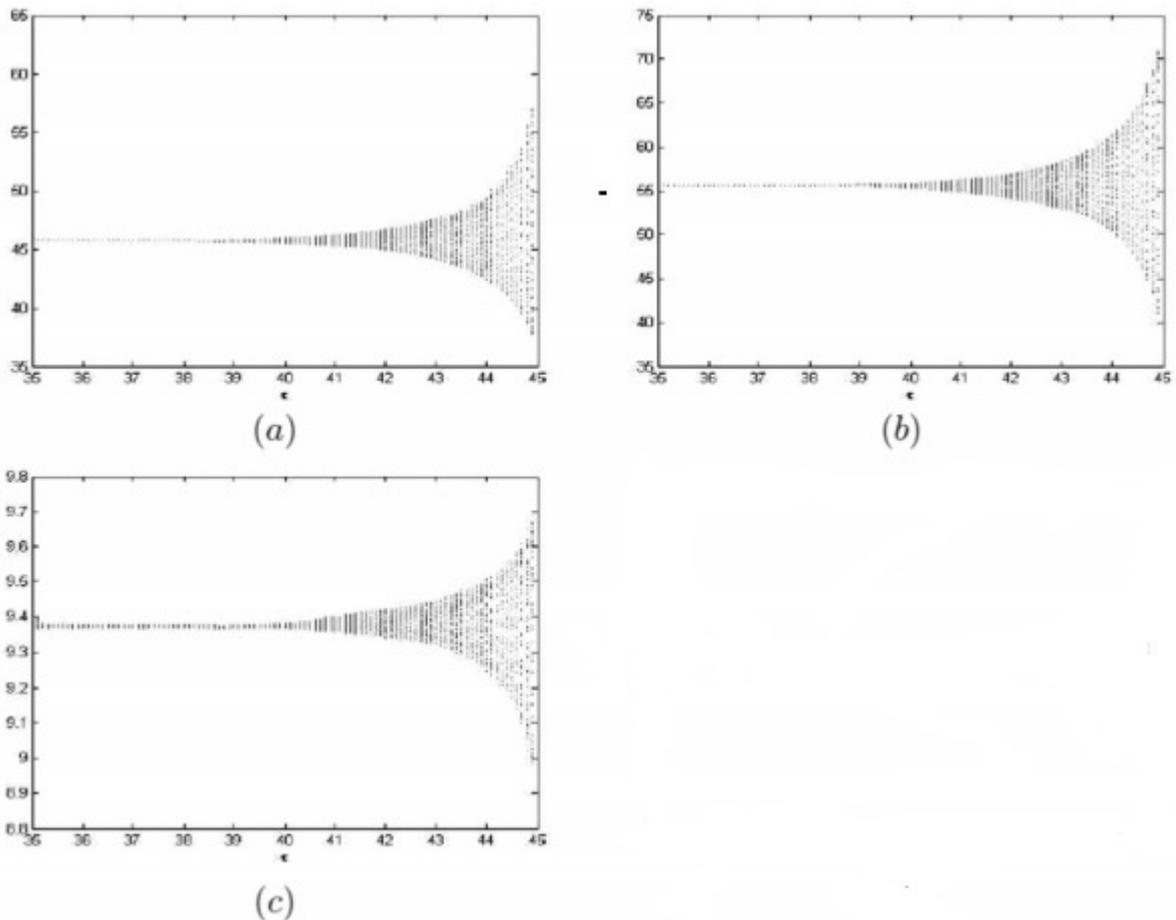
Figure 5: Bifurcation diagrams of system (1) with respect to  $\tau$  (a)  $S$ , (b)  $V$  and (c)  $I$
