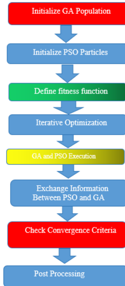
Figure 2: Work flow of GAPSO
